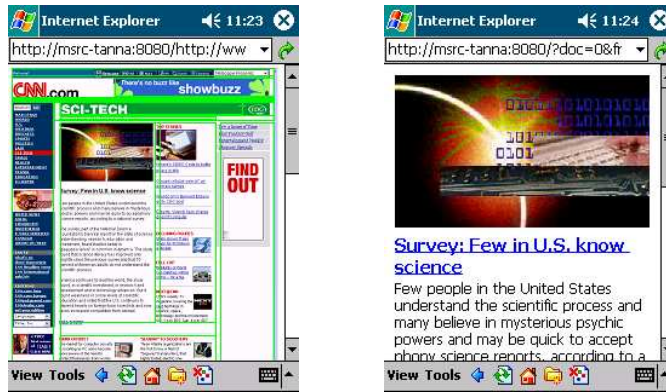
Figure 2: SmartView — overview of the page layout, with logical regions outlined in green (left), and direct access to the detail regions of the page (right).
